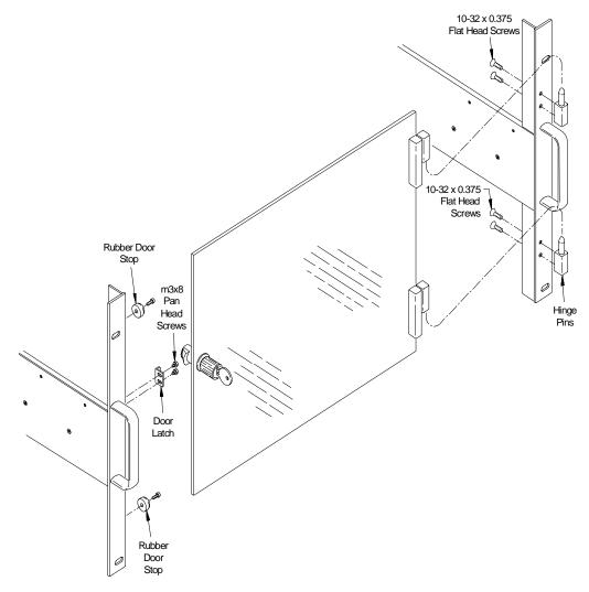
Figure 1. Installing the Acrylic Door Hinges, Door Stops, and Latch Keeper.
